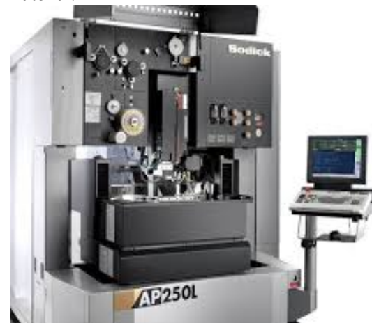
Fig. 7 Setup for Wire Cut Electro Discharge Machine
